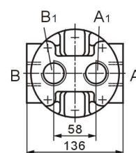
A,B,A<sub>1</sub>,B<sub>1</sub> Service line ports
