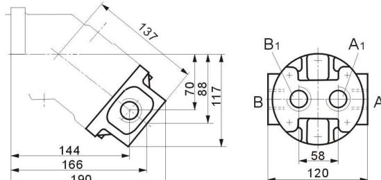
A,B,A<sub>1</sub>,B<sub>1</sub> Service line ports M27×2
