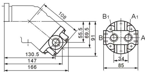
A,B,A<sub>1</sub>,B<sub>1</sub> Service line ports M22×1.5
