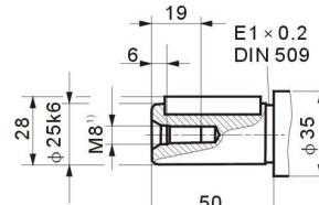
1) centering bore according to DIN 332
