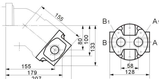
A,B,A<sub>1</sub>,B<sub>1</sub> Service line ports M33×2
