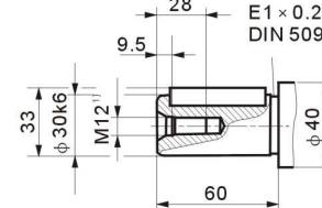
1) centering bore according to DIN 332 (thread according to DIN 13)
