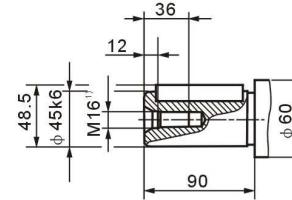
1) centering bore according to DIN 332 (thread according to DIN 13)
